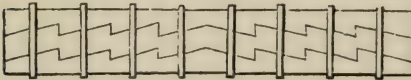
Fig. 87—Represents a solid built beam of three courses arranged with indentations and confined by iron hoops.
